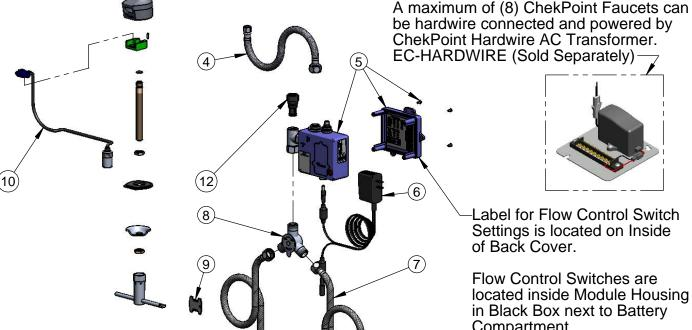
Label for Flow Control Switch Settings is located on Inside of Back Cover.
